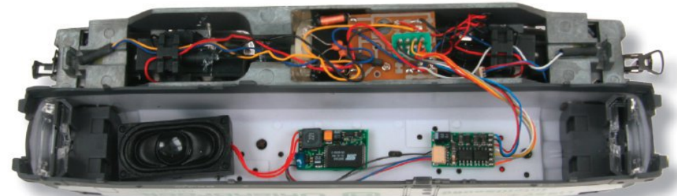
Decoder 76 420, Sound module 32 100 and loudspeaker 31 130 installed in a PIKO Taurus. See the parts.
